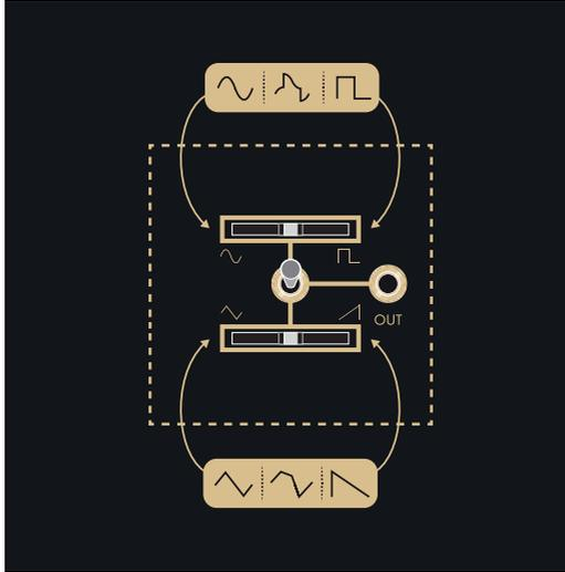
**Oscillator 1:** If the **Waveform Selection Toggle** is in the up position, the signal present at the **Waveform Output** will smoothly morph between a sine waveform and a triangle waveform as the **Waveform Crossfader** moves from left to right. If the **Waveform Selection Toggle** is in the down position, the signal present at the **Waveform Output** will smoothly morph between a ramp waveform and a square waveform as the **Waveform Crossfader** moves from left to right.
